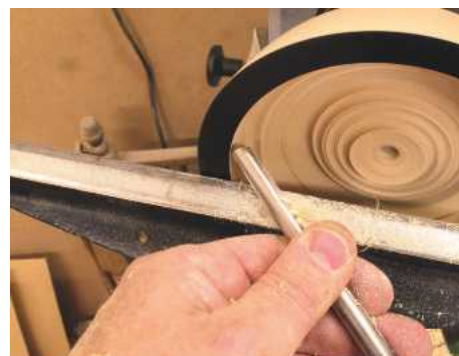
Pic.4 The small bowl gouge is the best tool for putting a slight undercut on the rim of your bowl as a scraper could tear the grain; this is not an easy technique but definitely one worth mastering
